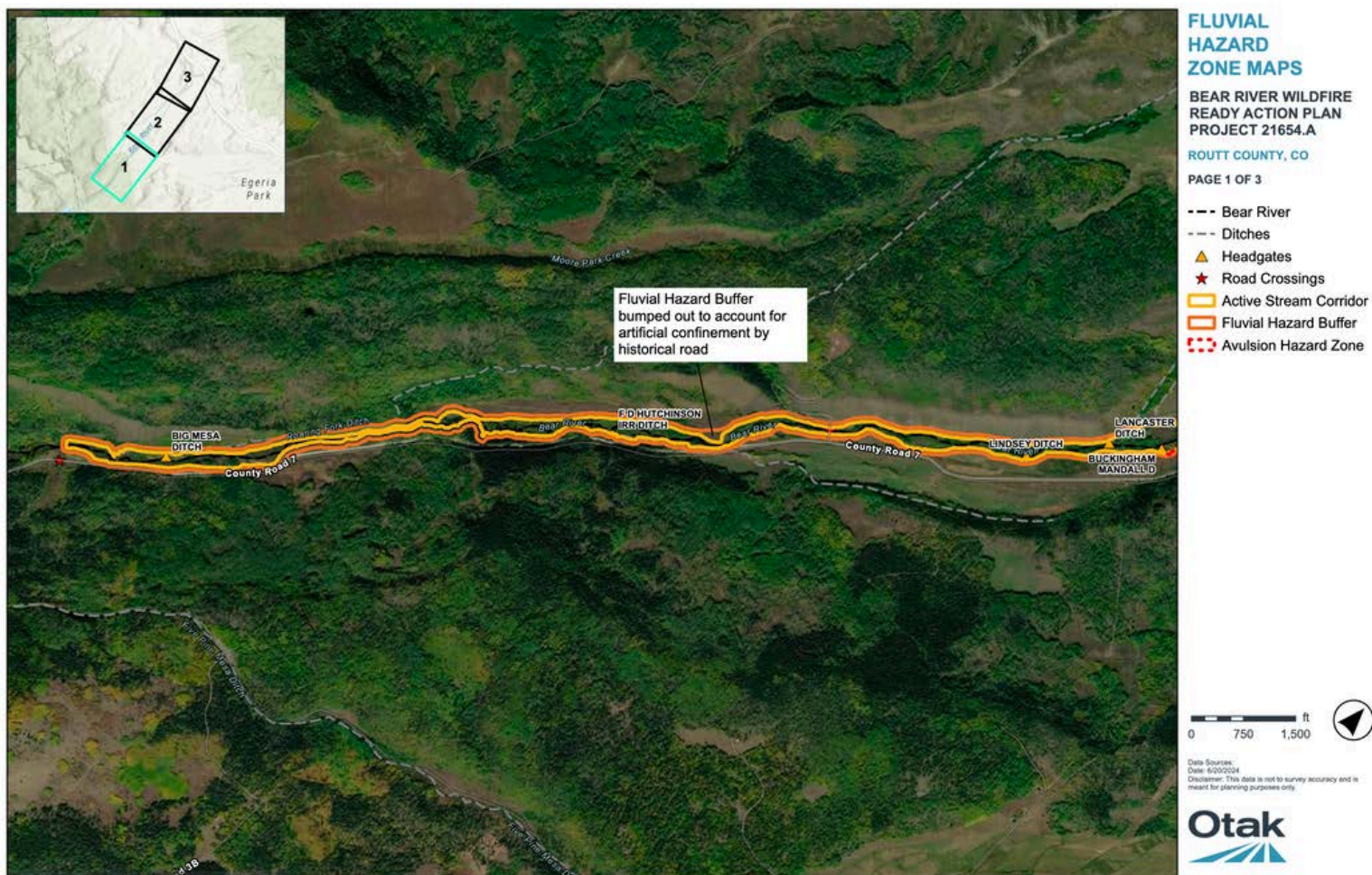
Map 16. Fluvial Hazard Zone Mapping for the Upper Sub-Reach of Bear River
